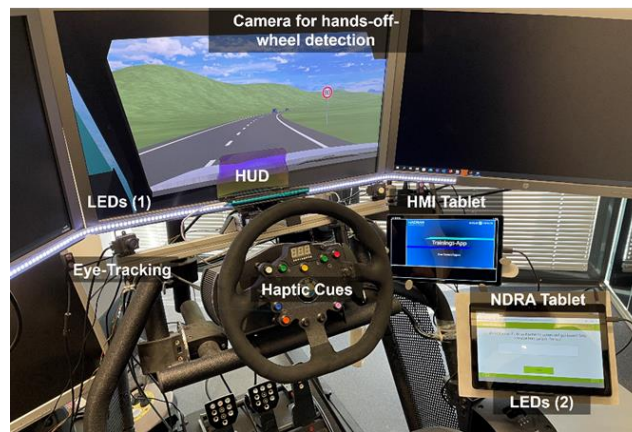
Figure 1 - Integrated fluid HMI components of the Virtual Vehicle holistic simulator study
