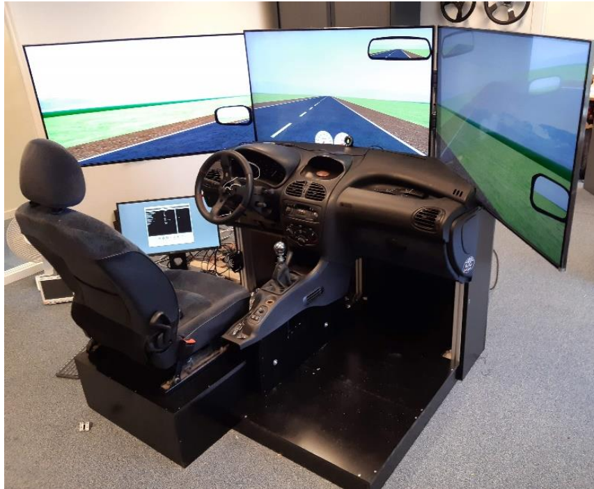
Figure 3 Car simulator developed by DriveSimSolutions, using OEM Peugeot 206 parts
