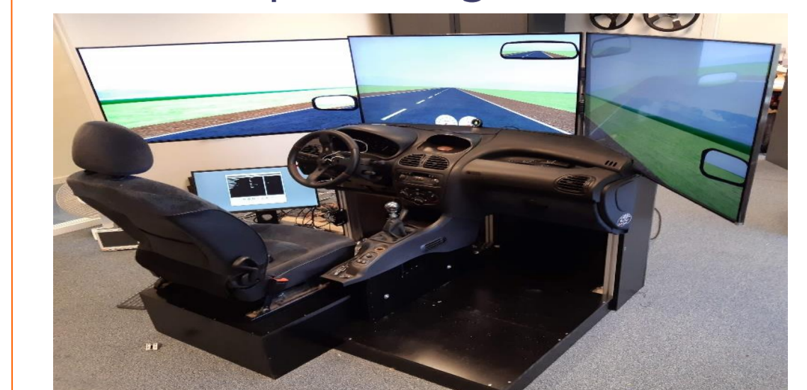
Figure 3: Car simulator developed by DriveSimSolutions, using OEM Peugeot 206 parts
