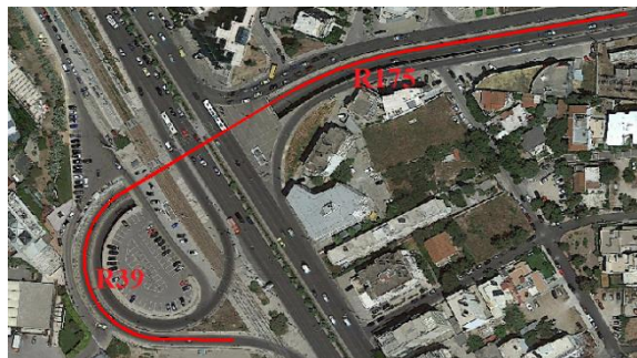
Image 5: Alimou Interchange, 175 and 39 meters radii horizontal curves (trumpet)
