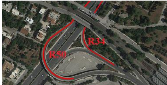
Image 3: Kimis Interchange, 34 and 50 meters radii horizontal curves (trumpet)
