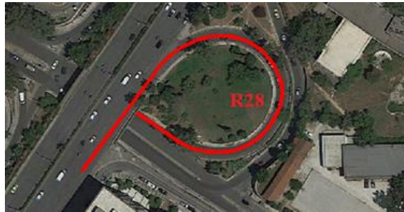
Image 2: Kifisias Interchange, 28 meters radius horizontal curve (clover section)
