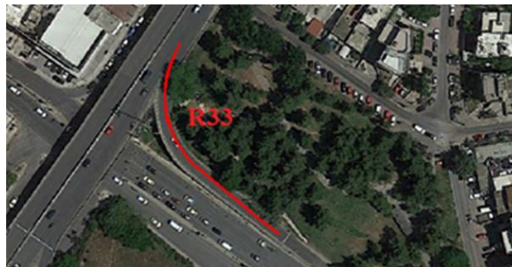
Image 4: Kapodistriou Interchange, 33 meters radius horizontal curve (diamond section)
